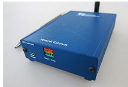
VEmesh Gateway for all types of networks (available also in DIN Rail case)
