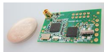
VEmesh Node module for VEmesh Extension to Lighting networks
