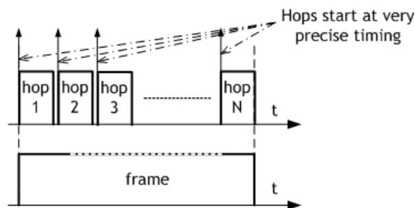
Figure 2 - The precise timing of the hops and the frame
