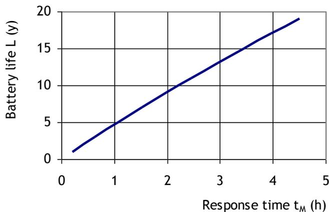
Figure 7 - Battery life versus the response time in the example
