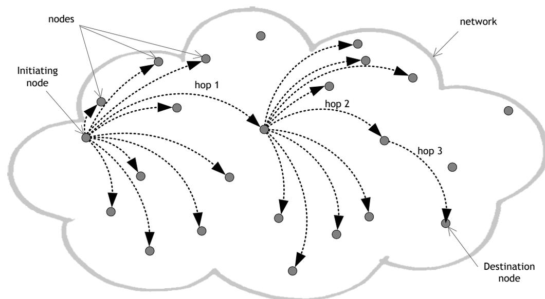
Figure 1 - In a mesh network, the messages propagate in hops
