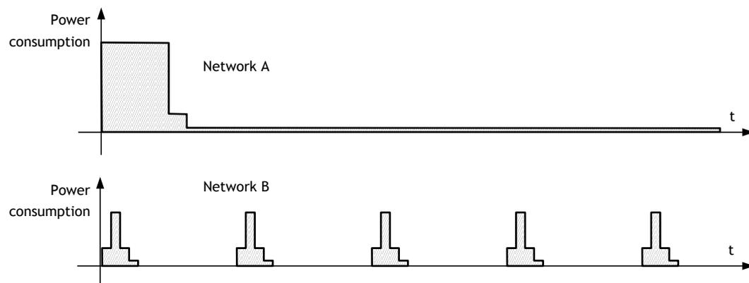
Figure 4 - Illustration of different power consumption patterns for Networks A and B
