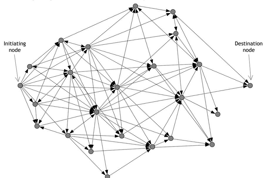
Figure 3 - Illustration of a 3-hop flooding based networks example
