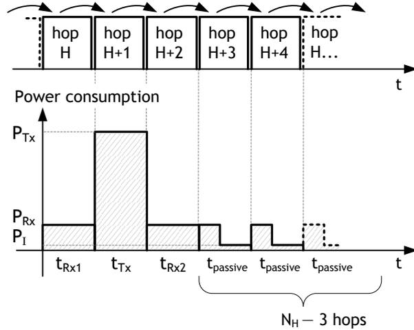
Figure 6 - The passive mode lasts  $N_H - 3$  hops and then the cycle starts again
